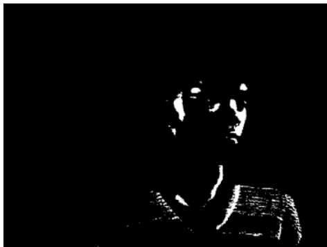
FIG 2.B RESULTING IMAGE AFTER APPLYING THRESHOLD FOR MOTION
